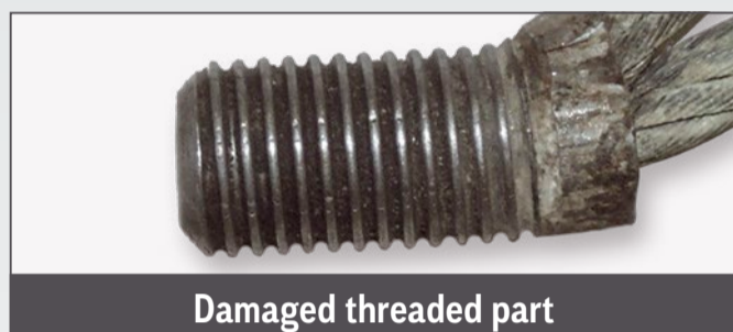
Loosening of external layer
