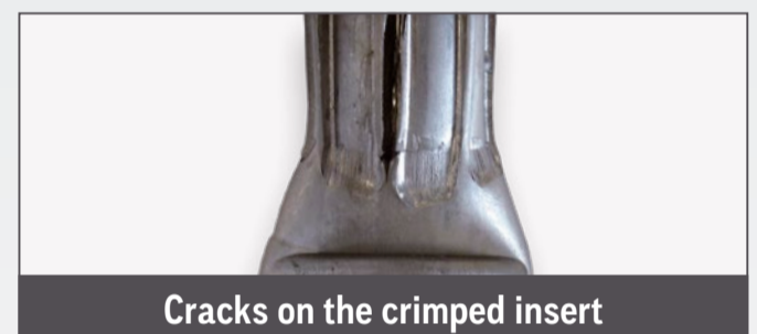
Pull-out of wire rope from crimped part
